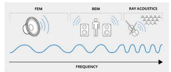
By combining boundary element, finite element, and ray acoustics analysis in a multiphysics environment, COMSOL 5.3a delivers unprecedented acoustic modeling capabilities.
