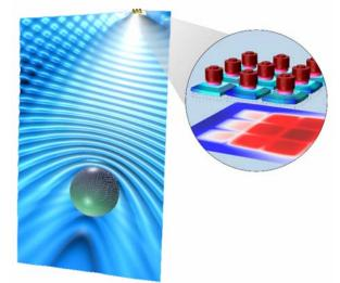
Scattering of acoustic waves generated by a piezoelectric tonpilz sonar array. Left: Sound pressure level. Right: Deformation of the array and generated total acoustic pressure field.
